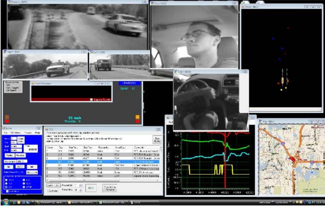
Fig. 2. Cabin instrumentation in the experimental vehicles including cameras and CAN signals.
