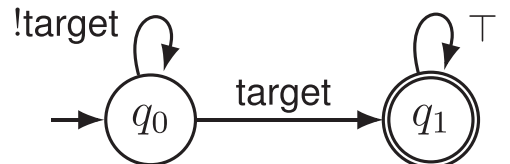
Figure 3. DFA \mathcal{A}_\phi for scLTL formula \phi = \Diamond target .
